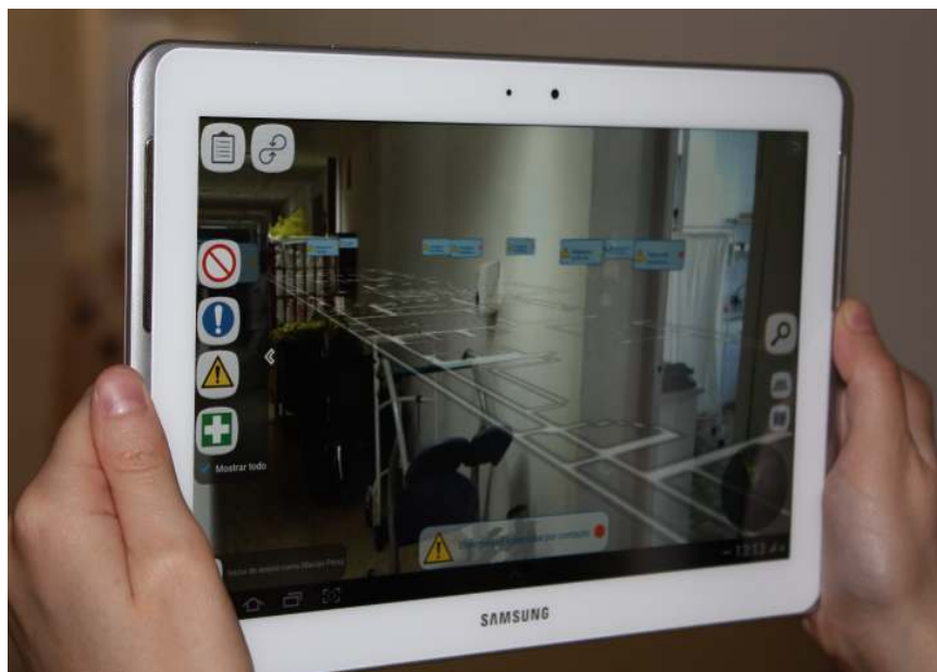
Figure 2. Emergency responders will use AR to find and follow the safest route through a building. Safety management operators will be prompted to manage a risk situation in real time (Image courtesy of Hopital La Magdalena and the ANGELS Consortium)
